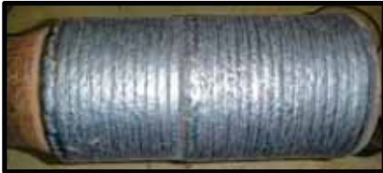
Re-built Tool Joint prior to machining
