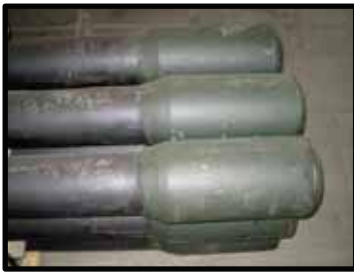
Re-built Tool Joints after machining
