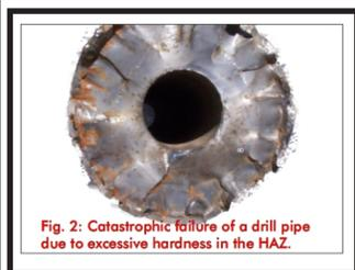
Fig. 2: Catastrophic failure of a drill pipe due to excessive hardness in the HAZ.
