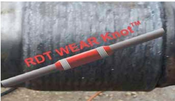
Figure 6. RDT wear knot with Coolbanding.
