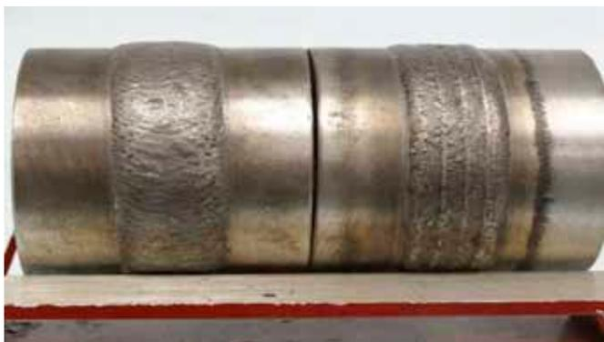
Figure 5. Comparison of conventional hardband to Coolband.
