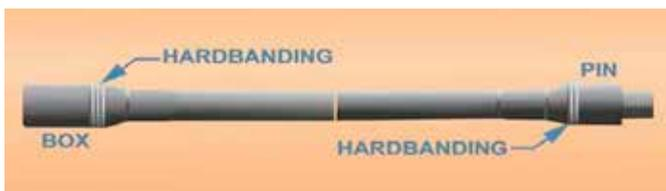
Figure 1. Drill pipe components.
