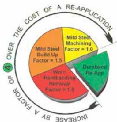
Figure 4. A pie chart illustrating the added costs incurred when hardbanding requires removal.
